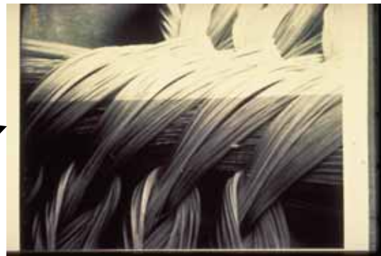
Magnification of tie yarns
